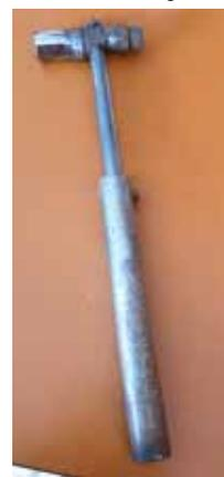
**Homemade 4-in-1 tool has 2 different size sockets, a punch, and a 16-in. long retractable handle that's used like a slide hammer to strike the punch.**
