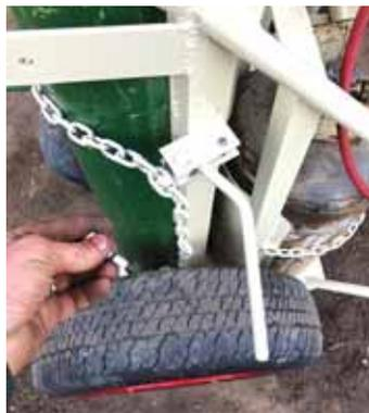
**A spring-loaded, over-center chain holds oxygen tank in place in the vertical position.**
