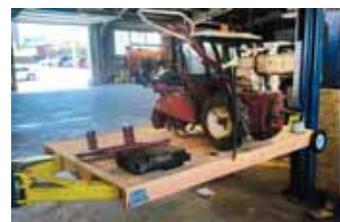
**Wooden platform rides up or down on a 2-post electric-hydraulic car lift, raising machines to a comfortable work height.**
