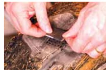
Glue-on patch can even fix punctures on a tire's sidewall.
