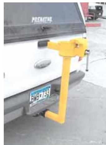
L-shaped steel arm has a round steel plate on top with holes in it to bolt on vise.
