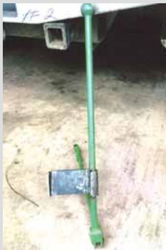
**Mike Peterson,** Bellingham, Wash.: "I welded a steel foot pad onto the bottom of the clutch lever on my 1953 John Deere 50 tractor. It lets me operate the clutch by just lightly pushing on the pad with my foot. I came up with the idea because while backing up to an implement it's hard to operate the clutch by hand, and look back at the same time. The foot-controlled clutch also frees up my hand to operate the 3-pt. lever."
