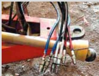
**Landen Boes,** Fostoria, Ohio: "We prevent wrong hookups of hydraulic hoses on our tractor by color coding each pair of hoses, spray painting them red, white and blue to match the tractor's number one, two, and three remote outlets. If we need to use a fourth outlet we paint those hoses green. We just paint an 8-in. long strip above each hose coupler. It's an easy way to tell at a glance where to plug the hoses in."
