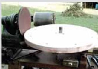
**Milan Hochstetler,** Cumberland, Va.: "After accidentally breaking the spokes on one of the wheels on my Montgomery Ward 20-in. band saw, I made a new one using 2 pieces of 3/4-in. thick plywood. I used Tite Bond III wood glue ([www.titebond.com](http://www.titebond.com); ph 800 669-4583) to fasten a rubber strip to the wood."
