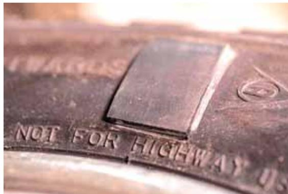
External tire patch glues on over puncture or slice in tubeless tire. You deflate tire and glue damaged portion back together, then use a special adhesive to apply patch.
