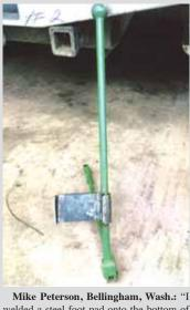
welded a steel foot pad onto the bottom of the clutch lever on my 1953 John Deere 50
