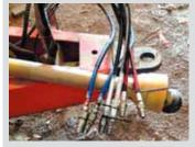
Landen Boes, Fostoria, Ohio: "We prevent wrong hookups of hydraulic hoses on our tractor by color coding each pair of hoses, spray painting them red, white and blue to match the tractor's number one, two, and three remote outlets. If we need to use a fourth outlet we paint those hoses green. We just paint an 8-in. long strip above each hose coupler. It's an easy way to tell at a glance where to plug the hoses in."
