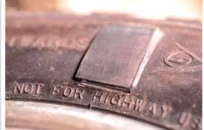
External tire patch glues on over puncture or slice in tubeless tire. You deflate tire and glue damaged portion back together, then use a special adhesive to apply patch.
