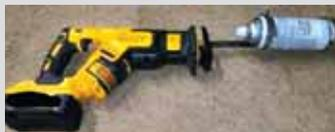
**Glenn A. Haley, Andover, N.H.:** “A quick and easy way to thoroughly shake a spray paint can is to attach it to the blade in a reciprocating saw. Just use a couple hose clamps to hold the can on the blade and insert
