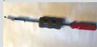
**James Nicholson, Lisbon, Ohio:** “I work on small engines and had need of a puller to remove an exhaust valve seat. I had recently been to a local garage sale and I purchased some small gear puller legs. I decided I could make a puller out of one. I cut one leg in half and welded it into a 3/8-in. threaded bolt coupler. Now it screws onto my seal puller and works great.”
