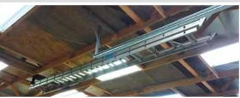
Extension ladder is suspended horizontally below shop loft when not in use, and is hinged at one end. It can be lowered to floor by releasing a rope tied to a boat cleat mounted on shop wall.
