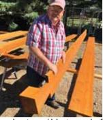
Waite used homemade chainsaw jig to produce trapezoidal cuts on ends of boards he used for siding his house. Boards interlock at corners of house.
