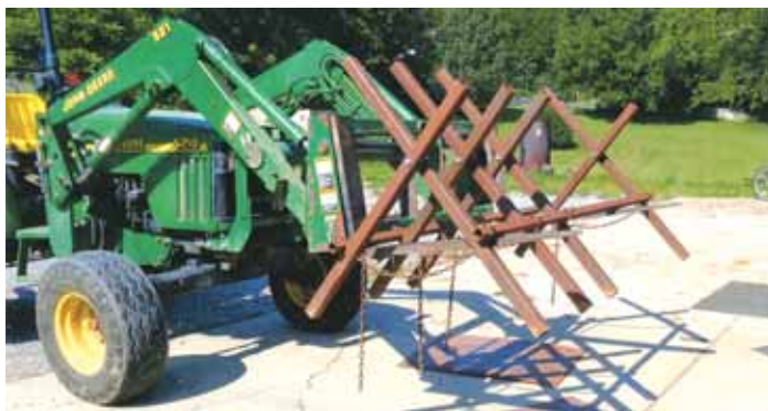
Mariner transports freestanding steel sawhorse on his tractor's loader forks. Sawhorse quickly folds up out of the way for storage.
