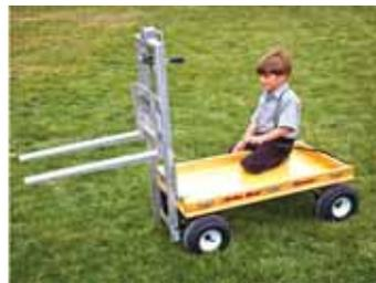
Aluminum forklift has 24-in. forks and is designed to attach to a child's wagon or pedal tractor. Operator hand-cranks forks up or down.
