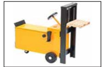
Forklift with rear caster wheel relies on leg power to move and turn. Turning a crank raises and lowers the mast.
