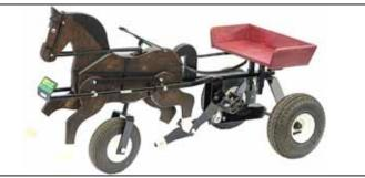
Ride-on wooden cart operates like a tricycle. When you pedal, the horse's four legs move. Reins are used to steer.
