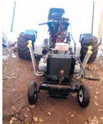
Denny Brookins used the 100 hp. engine off a motorcycle to power his home-built pulling tractor.
