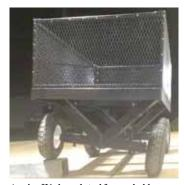
A pair of V-shaped steel frames hold wagon level as axles pivot.
