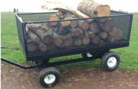
Cart's front and rear axles pivot independently from side to side, thanks to Kuenzi's home-built suspension system.
