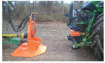
Combi Hitch comes in 2 parts that attach to implement and tractor. Electrical and hydraulic connections, along with the pto shaft, connect as tractor backs up.
