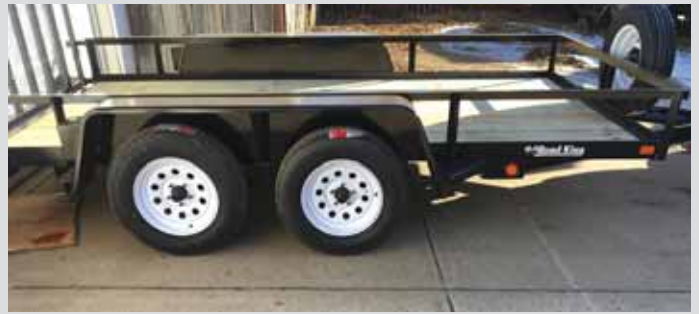
Gary Swensen's custom-built 12-ft. trailer has a rear hitch, steps on the side, tandem axles, brakes, and extra rear lights, along with a heavy-duty ramp and rear bumper.
