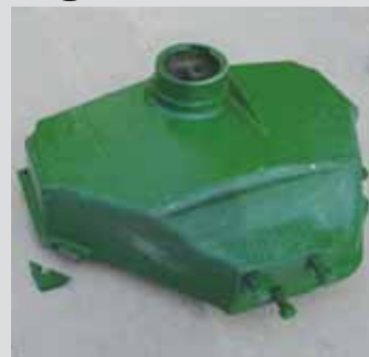
John Ottem had a professional weld this broken cast iron radiator back together, using Magna 770 rod for welding cast iron. He then drilled a hole through the weld.
