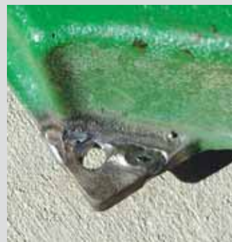
John Ottem had a professional weld this broken cast iron radiator back together, using Magna 770 rod for welding cast iron. He then drilled a hole through the weld.
