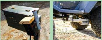
A throttle cable is attached to upright tube, along with a steering control switch connected electronically to a linear actuator on rig's steering axle.
