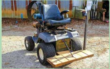
Moller started with an old Craftsman mower to build his powered cart, reversing the direction of the machine and adding a footrest platform on front.
