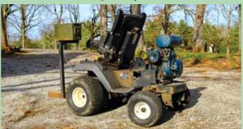
He mounted a seat over mower's former rear axle and a Kohler engine over the former front axle. Upright steel tube with controls at the top mounts on platform.
