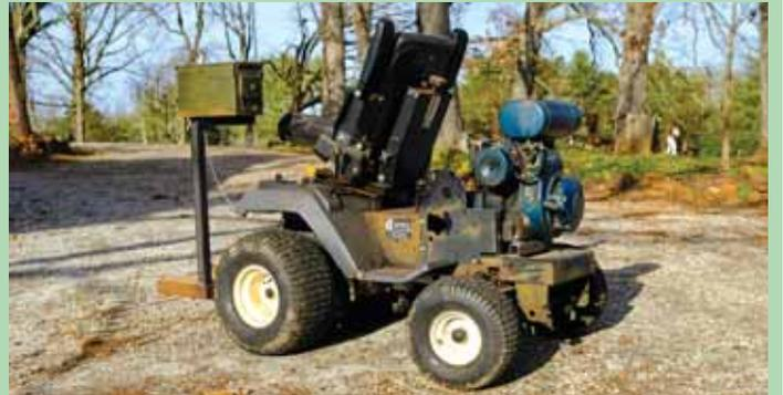
He mounted a seat over mower's former rear axle and a Kohler engine over the former front axle. Upright steel tube with controls at the top mounts on platform.
