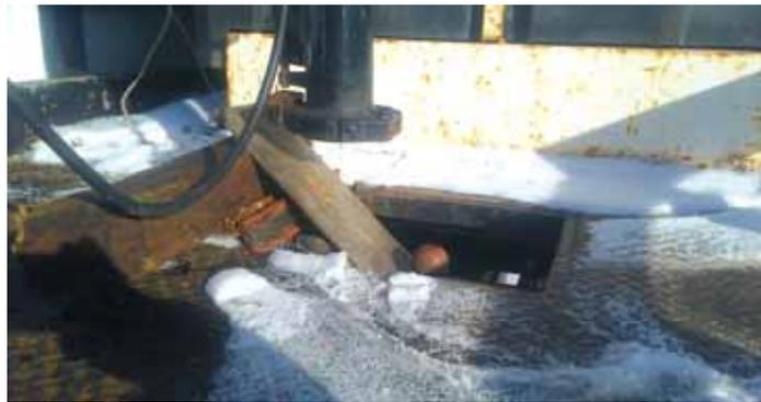
Lower end of steel plate sets against base of ball in truck bed, while upper end rests against a wood block. As trailer is lowered, gooseneck slides along plate and onto ball.
