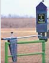
**Bale Cracker** – Nifty new bale handler has a built-in slicer that cuts off twine, net wrap or plastic wrap, all without you having to leave the tractor seat. The patented slicing mechanism consists of common sicklebar mower blades built into one arm that cut the wrapping and then lift it away as the bale drops, eliminating the chance for any of the material being ingested by livestock. ([www.maxilator.com](http://www.maxilator.com); ph 866 429-2253)
