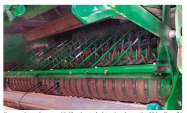
Compression rack comes with 10 rods attached to a long bar made of 8-in. dia. solid steel tubing.
