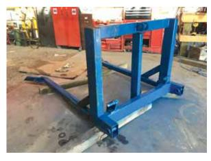
McNally built these 3-pt. bale forks using part of the frame and forks off an old Brandt self-loading bale processor.
