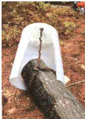
**Log is secured by a choker chain that runs through hole in bottom of plastic cone.**
