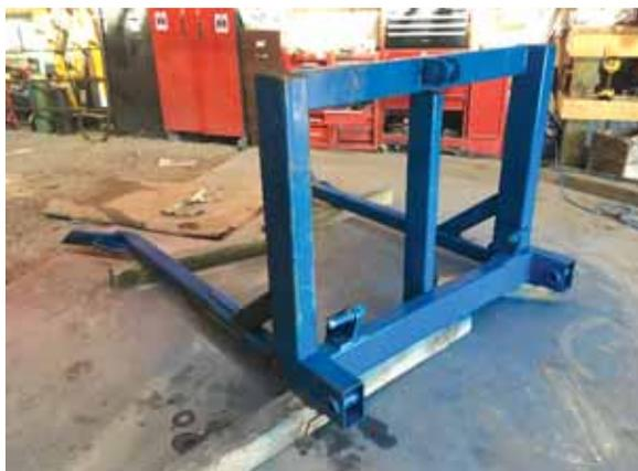
**McNally built these 3-pt. bale forks using part of the frame and forks off an old Brandt self-loading bale processor.**
