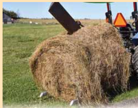
Combination carrier and cutter slices round bales in half for grinding by a TMR mixer.
