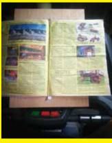
I made a device to make it easier to read FARM SHOW while walking on my treadmill. It was difficult to find a place to put the magazine since the pages are floppy. So I made a support out of a piece of plywood with a coat hanger down the middle that goes through the center of the pages. There's a block of wood attached to the back that acts as a hanger at the top of the treadmill. Reading FARM SHOW makes the exercise minutes go much faster! (Michael Heron, Lloydminster, Sask., Canada)
