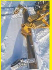
To keep from scraping rocks off my driveway when moving snow with my grader blade, I installed two heavy-duty 12-in. swivel caster wheels, one at each end of the blade. I use the third link to adjust the height before I start clearing the driveway. (Richard Mountcastle, Rockville, Ind.)
