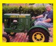
My 1/4-scale John Deere D was built totally from scratch. It's powered by a Deere pony motor and Cub Cadet rear end. It has a functional belt pulley, flywheel, pto and hand clutch. I made the fenders and all the sheet metal parts, except the hood, which was made by my friend, Myron Hoelscher. The radiator core was special-ordered. The rear wheels are cut down dump rake wheels and the front wheels came off a cultivator. The seat is an original Deere cast iron seat.
