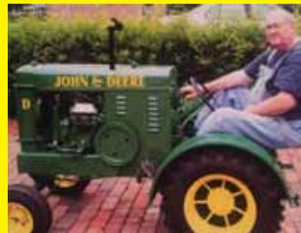
My 1/4-scale John Deere D was built totally from scratch. It's powered by a Deere pony motor and Cub Cadet rear end. It has a functional belt pulley, flywheel, pto and hand clutch. I made the fenders and all the sheet metal parts, except the hood, which was made by my friend, Myron Hoelscher. The radiator core was special-ordered. The rear wheels are cut down dump rake wheels and the front wheels came off a cultivator. The seat is an original Deere cast iron seat.
