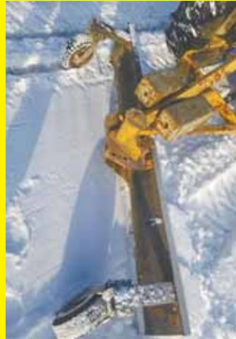
To keep from scraping rocks off my driveway when moving snow with my grader blade, I installed two heavy-duty 12-in. swivel caster wheels, one at each end of the blade. I use the third link to adjust the height before I start clearing the driveway. **(Richard Mountcastle, Rockville, Ind.)**
