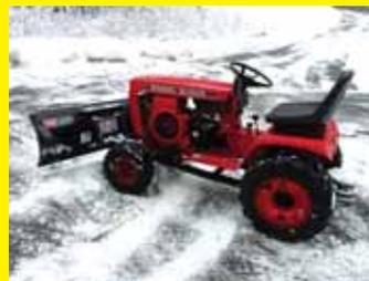
I replaced a rusted-out 48-in. plow blade on my old C-120 Wheel Horse tractor with a ProVantage 50-in. blade I bought at Amazon.com for a couple hundred dollars. The blade came with trip springs, skids and a wear bar. It was easy to adapt it to the existing plow frame with no welding and only some minor drilling. The new blade is very strong, made from 12-ga. steel. **(Lee Murgia, Pelham, N.H.)**
