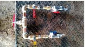
U-shaped splitter valve hooks up to an air compressor, allowing Greff to activate and deactivate his semi trailer air brakes from anywhere around the trailer.
