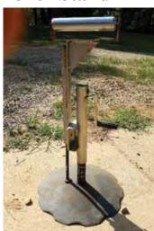
Johnson built several of these home-built trailer jack "roller stands", which he uses with his band saw to handle long material.
