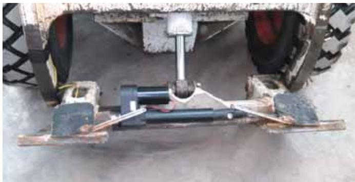
**Electric actuator eliminates the need to manually lock and unlock skid loader's quick-attach levers.**
