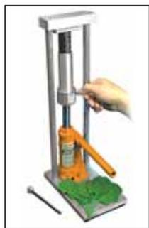
**A variety of sap sensors detect plant nutrient levels, including an electrical conductivity meter (above). A hydraulic plant sap press is shown at left.**
