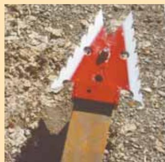
**V-shaped steel "cutting teeth" slide onto tips of skid loader forks.**
