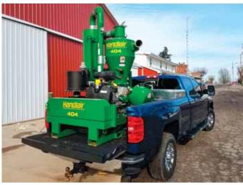
Compact grain vac is small enough to mount in a pickup with a skid loader. It's available in either electric or gas-powered models.
