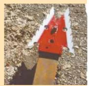
V-shaped steel "cutting teeth" slide onto tips of skid loader forks.
