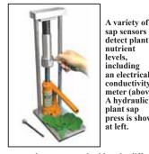
detect plant nutrient levels, including an electrical conductivity meter (above). A hydraulic plant sap press is shown at left.
