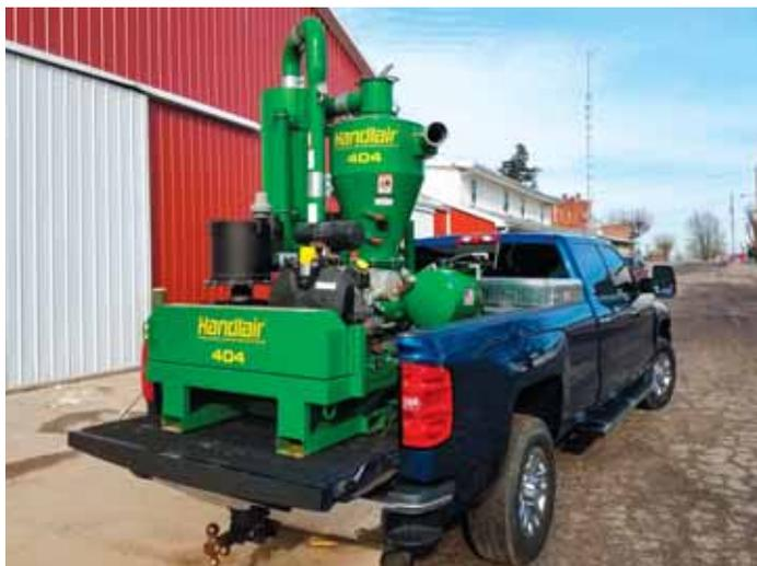
**Compact grain vac is small enough to mount in a pickup with a skid loader. It's available in either electric or gas-powered models.**
