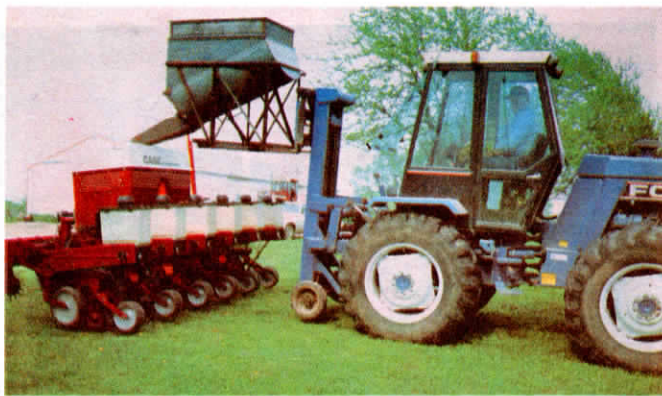
Schild mounted Gleaner hopper on angle iron frame that he handles with forklift.
