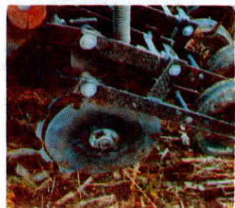
Double disc opener consists of a serrated disc and a smooth-edged disc, with the serrated blade leading by about an inch to cut through residue.
