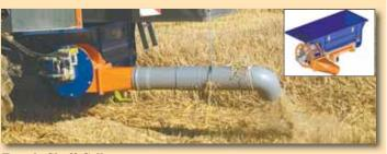
French Chaff Collector - Two-stage hydraulic-powered chaff collector catches crop material in a hopper, then augers it over to an impeller that can either blow chaff into a trailing wagon, or drop it in a windrow behind the combine.www.menuepaille.fr
