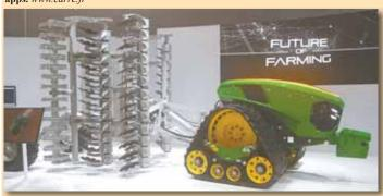
Deere's Autonomous Tractor - Code-named "Joker" while under development, Deere's electric-powered robot tractor runs on two sets of tracks. Developed in Germany, it puts out 250 kW through the tracks and another 250 kW on the implements. The tricky part is that it's powered by cables that can be laid out in the field or carried by a second carrier vehicle.
