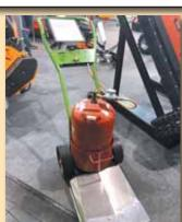
One-Row Flame Weeder - Propanepowered weed burner from the Netherlands has a low profile to take out weeds under plant canopies or near obstacles around the farmyard. Designed to be very easy to maneuver, the weight of the gas tank is directly over the wheels. https://www. onkruidbrander.com/en/thermhit/
