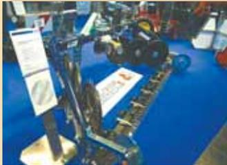
**New Double Knife Design** - ESM introduced a new double-knife cutterbar, a totally new design that reduces wear and the formation of gaps between blades. It eliminates the need for regrinding all cutting edges of the blades, and new-style mounts hold more securely. [www.esm-ept.de](http://www.esm-ept.de)
