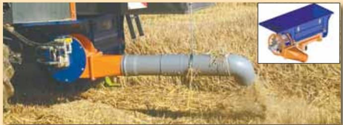
**French Chaff Collector** - Two-stage hydraulic-powered chaff collector catches crop material in a hopper, then augers it over to an impeller that can either blow chaff into a trailing wagon, or drop it in a windrow behind the combine. [www.menuepaille.fr](http://www.menuepaille.fr)
