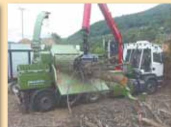
**Giant Wood Chipper** - Big drum-type chipper swallows whole trees, quickly turning them into compostable chips. The innovative Italian company makes a wide range of chippers, wood processors, and other related wood handling equipment. [www.pezzolato.it](http://www.pezzolato.it)
