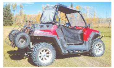
Brian Dickinson uses straps and a load binder to attach home-built, fold-up trailer on back of his 4-wheeler.
