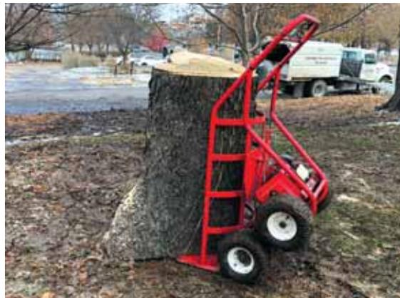
Motorized cart rides on 4 wheels – 2 free-spinning wheels followed by 2 drive wheels. Operator tilts cart back to engage the drive wheels.
