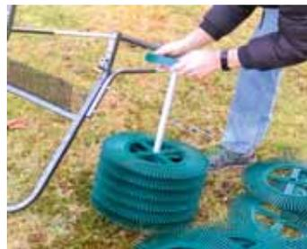
**Spacers are installed by pulling a hinge pin from each end of Cyclone Nut Rake axle and sliding pickup wheels off.**
