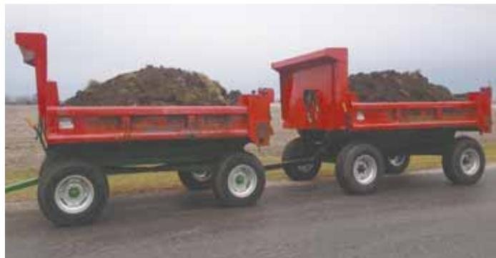
**Timm and Terry Johnson mounted “contractor” truck boxes on heavy-duty Deere running gears. The low-profile boxes carry heavy loads of dirt, concrete, firewood, and other materials. Because of the way the hoist is attached to the subframe, the front end of running gears do not lift up when the boxes are dumped.**
