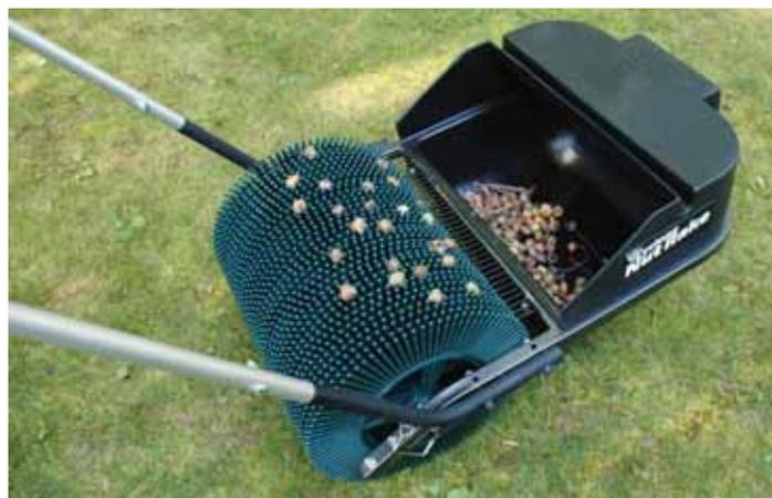
“It lets you gather all different sizes of nuts, by adding or removing detachable spacers between the pickup wheels,” says Matthew Coz about the new Cyclone Nut Rake.
