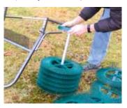
Spacers are installed by pulling a hinge pin from each end of Cyclone Nut Rake axle and sliding pickup wheels off.
