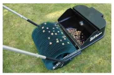
"It lets you gather all different sizes of nuts, by adding or removing detachable spacers between the pickup wheels," says Matthew Coz about the new Cyclone Nut Rake.
