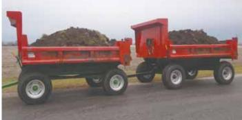
Timm and Terry Johnson mounted "contractor" truck boxes on heavy-duty Deere running gears. The low-profile boxes carry heavy loads of dirt, concrete, firewood, and other materials. Because of the way the hoist is attached to the subframe, the front end of running gears do not lift up when the boxes are dumped.
