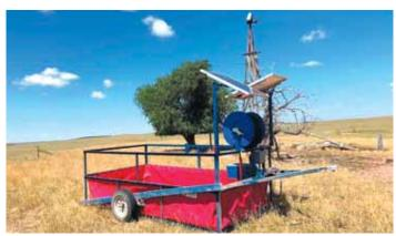
Mobile water tank mounts on its own trailer and comes with a float system and optional solar-powered pump.
