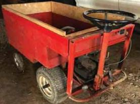
cart" was made using parts from a nair of riding mowers. Operator pulls back on
