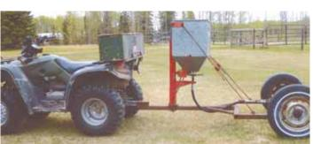
Dickinson mounted a Cyclone seeder on the wheels and axle off an old Toyota car. The axle's differential is used to drive the seeder's fan.
