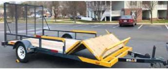
To return trailer to its original length, the operator uses a lever to break the plane on the extendable floor. He then applies the trailer brakes to lock the wheels, and backs up until trailer is compressed to its original length.
