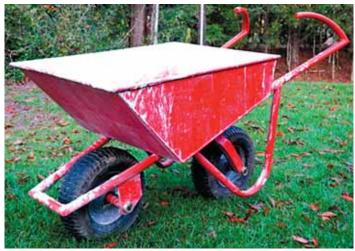
A second in-line wheel on the BeastBarrow helps carry heavy loads. Wheel is free to swivel, which makes it easier to push the load around curves.
