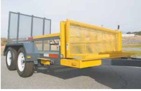
Extendable frame rides on a pair of telescoping steel tubes that are free to slide back and forth on rails.
