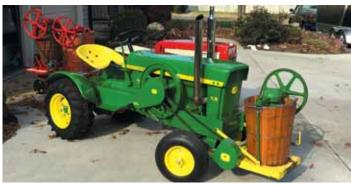
Riffey converted this Deere 140 garden tractor to look like a 1960's Deere 110, repowering it with a Deere 1 1/2 hp. hit and miss engine that belt-drives a 2-gal. ice cream freezer
