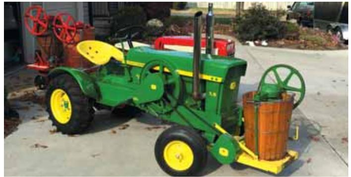
Riffey converted this Deere 140 garden tractor to look like a 1960’s Deere 110, repowering it with a Deere 1 1/2 hp. hit and miss engine that belt-drives a 2-gal. ice cream freezer on front of tractor.
