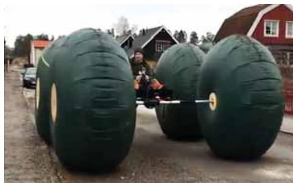
Amphibious vehicle has inflatable wheels that run on power tool motors. It travels at speeds up to 18 mph on land.
