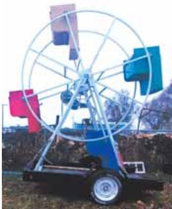
Portable mini Ferris wheel has 4-ft. wide seats and rides on a trailer chassis.
