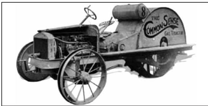
This shot of the Common Sense 8-cylinder tractor is unusual because most photos of the tractor show its right side. Here, the photographer put the focus on the engine, magneto, governor and carburetor, all easily accessible.
