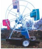
Portable mini Ferris wheel has 4-ft. wide seats and rides on a trailer chassis.
