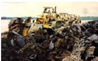
It took four D8 and D9 Caterpillar dozers linked together with cables and chains to pull the plow.
