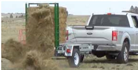
Remote-controlled, hydraulic bale pusher feeds big square bales back to twin vertical flakers.
