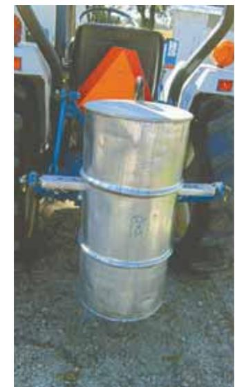
Concrete-filled barrel contains an embedded drawbar that attaches to 3-pt. lift arms.
