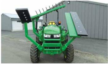
Push-up blade pushes feed back to where cattle can easily reach it. Groomer and pushup blade can be mounted on a single tractor to do double duty.
