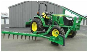
Tractor-mounted groomer uses hardened tines to "fluff up" bedding material and level it. An adjustable guide makes it easy for operator to follow the curb.
