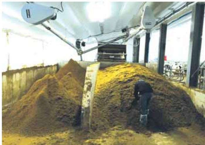
VYF manure digester separates nutrient-heavy liquids from undigested fiber. The dried material can be reused as bedding.
