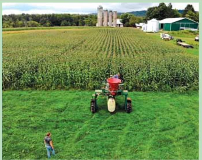
Jim Kreger removed the booms from an old Deere Hi-Boy self-propelled sprayer and mounted a spin spreader on the boom’s lift arms (above). Spreader raises 10 ft. high, allowing seed to launch across top of standing corn.
