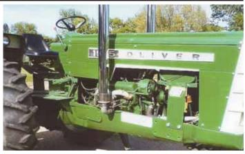
With a little help from a driveline fabrication shop, Bill Knutson repowered this Oliver 1555 tractor with a Chevy 350 engine.
