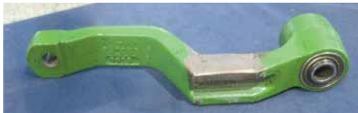
Rebuild kit improves the performance of old and worn parallel linkage arms by replacing the original bushings with sealed bearings.
