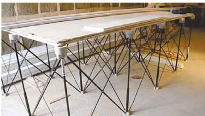
Portable workbench quickly folds out to provide a 4 by 8-ft. work surface.
