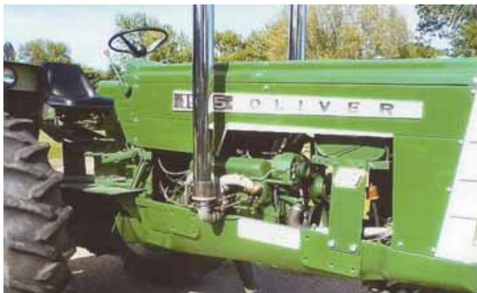
With a little help from a driveline fabrication shop, Bill Knutson repowered this Oliver 1555 tractor with a Chevy 350 engine.
