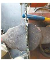
"I put the bar in the vise and run the file 3 or 4 times on each tooth, then move the chain ahead," he says.
