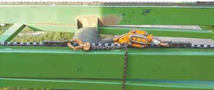
To pull his trailer’s floor chain tight again, Lacey made a pair of 8-in. long “fish hooks”. An eyelet welded onto one end attaches to hook on chain hoist.
