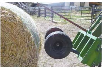
Two-wheeled unroller fits onto a pair of 2-ft. long stabilizer bars on loader-mounted bale spear.
