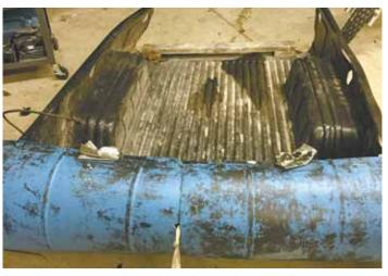
Setcoski cut a 55-gal. plastic barrel in half lengthwise to make 2 halves, then bolted them on front of plastic pickup bed liner.
