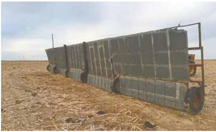
Barker uses old 60-ft. wide, 5-section Noble cultivators to make portable windbreaks that can be easily moved. Corrugated tin sheets bolt onto cultivator frame.
